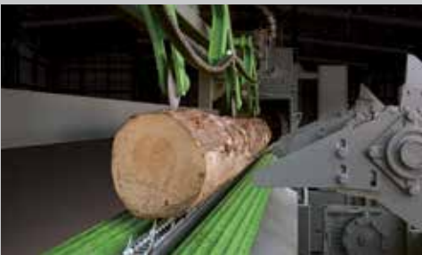
Infeed with log turning rollers
