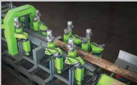
High throughput continuous infeed
