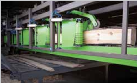
Auto. outfeed with separation of boards and waste
