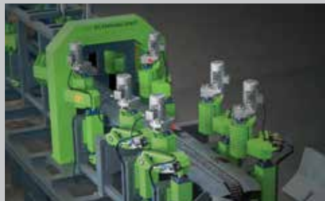
Scanning of logs with optimi- sation
